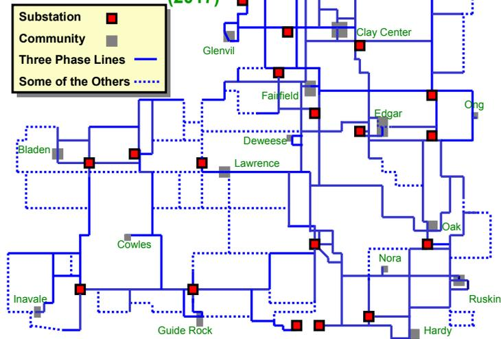
Like the transmission system, we have established tie-lines within our distribution system. Tie-lines represent less than 10% of the total miles of distribution line in service. Showing the other 90% of the distribution lines in service would make the map unreadable at this scale.
