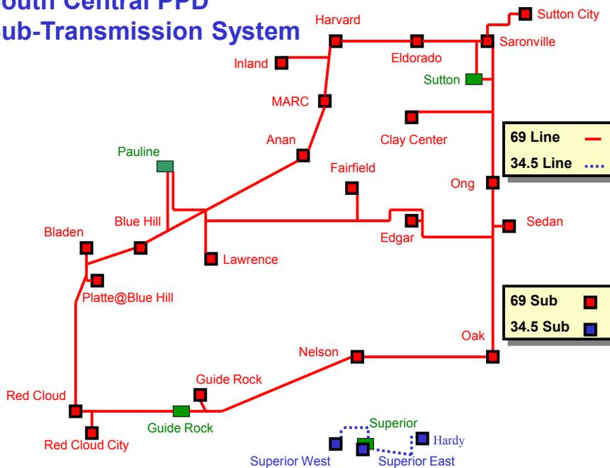
The drawing implies that all of the red lines are tied together. That is true mechanically, but not electrically. Power flows **from** an NPPD substation into our transmission system on through our distribution system **to** your meter.
